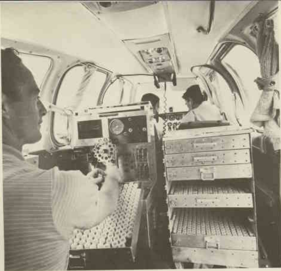
Aerial incendiary operation—with the priming and timing device in the foreground. On the flight deck are the pilot and a Forests Department officer who does the plotting and navigating.
