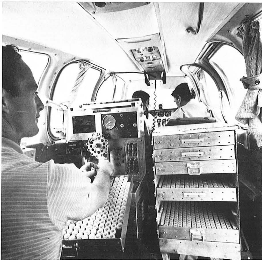
Aerial incendiary operation—with the priming and timing device in the foreground. On the flight deck are the pilot and a Forests Department officer who does the plotting and navigating.
