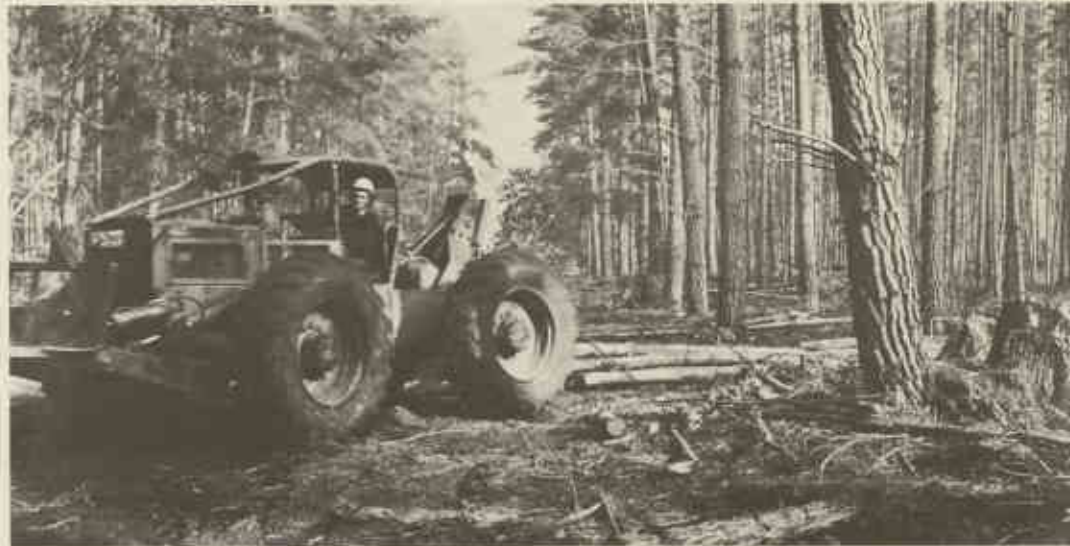
Selective logging in the Grimwade pine forest (above). Logs are snigged to a central point for cutting to length and loading on to log trucks.
