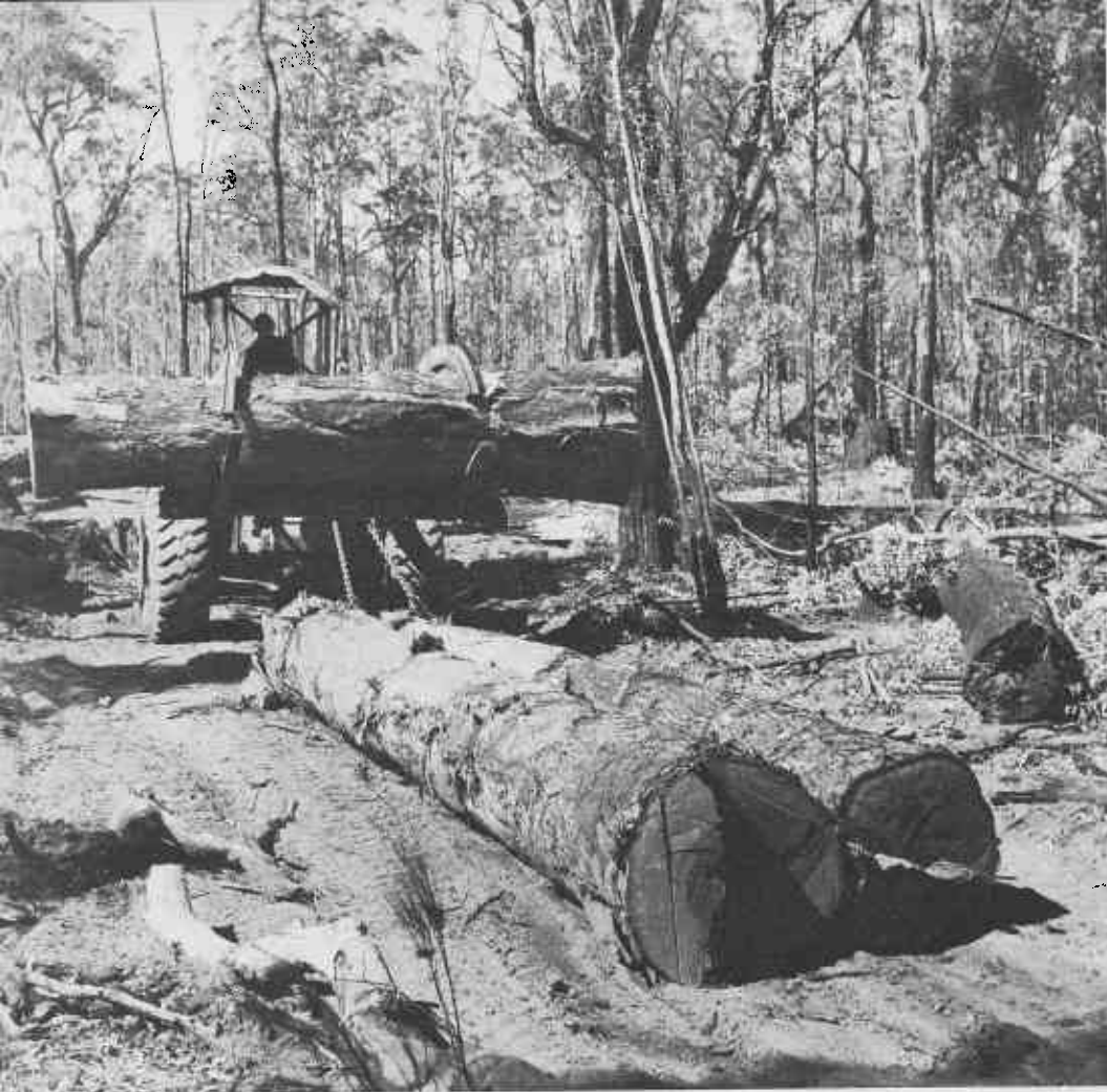
A modern logging machine, the rubber-tired tractor carries one jarrah log and snigs two behind (above), and doubles as a loading machine (below).
