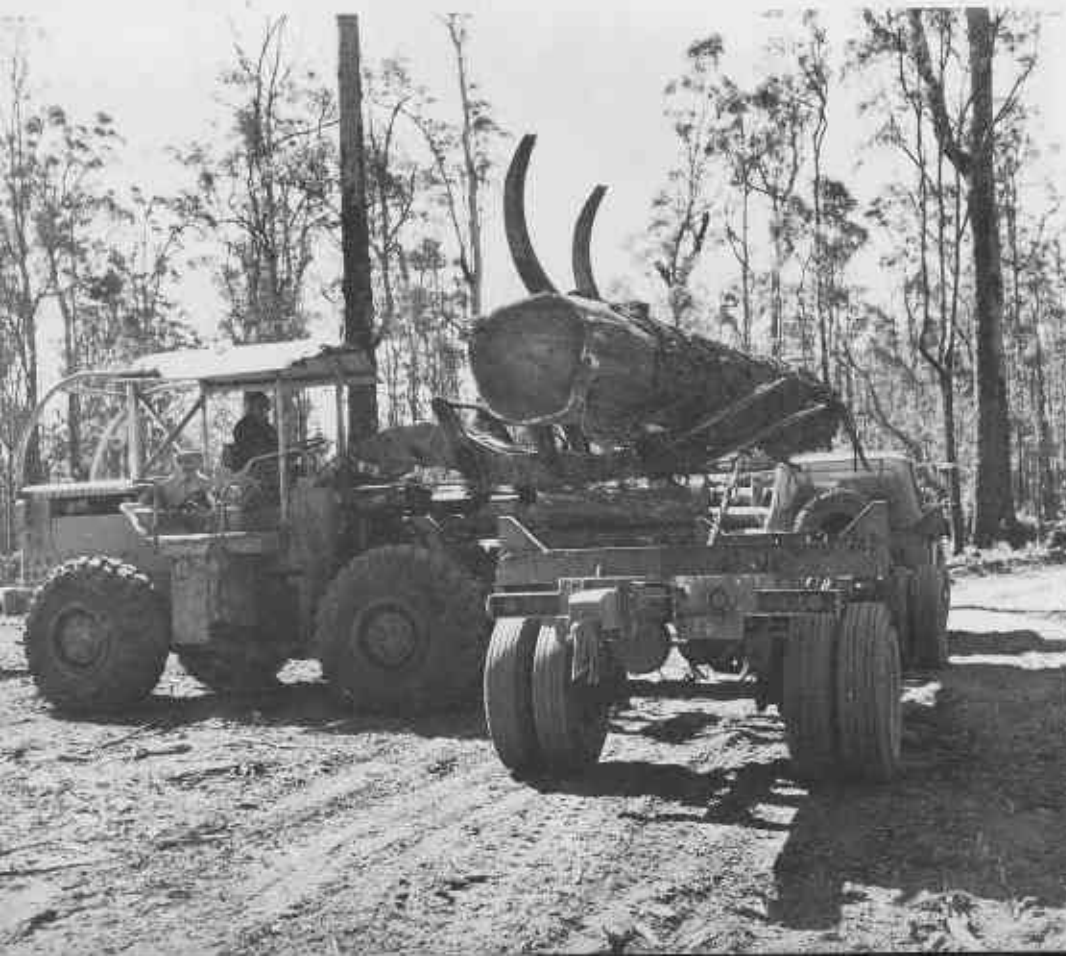
A modern logging machine, the rubber-tired tractor carries one jarrah log and snigs two behind (above), and doubles as a loading machine (below).
