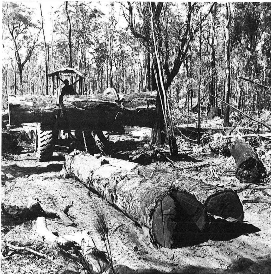
A modern logging machine, the rubber-tyred tractor carries one jarrah log and snigs two behind (above), and doubles as a loading machine (below).
