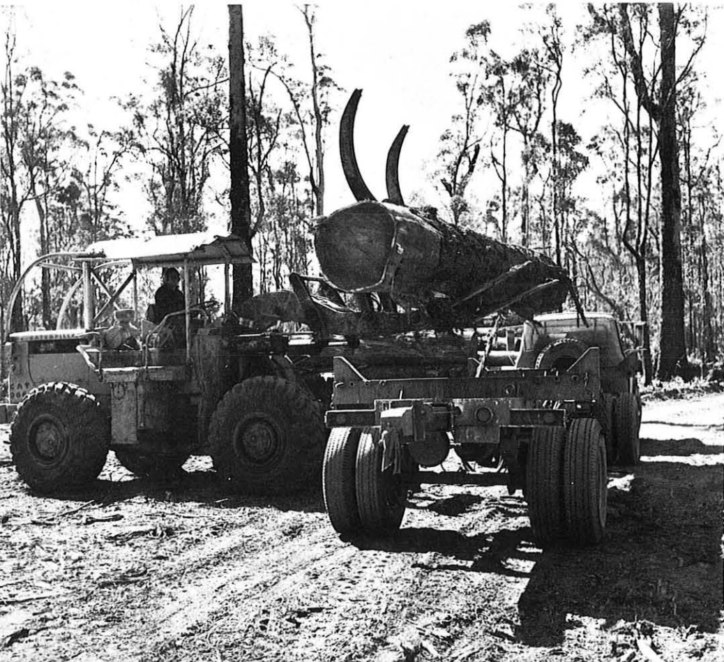
A modern logging machine, the rubber-tyred tractor carries one jarrah log and snigs two behind (above), and doubles as a loading machine (below).
