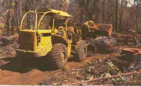
◀ Laboratory testing of soil carried on logging equipment which had been working in a dieback area showed that it contained P. cinnamomi . (Govt. Photographer)
