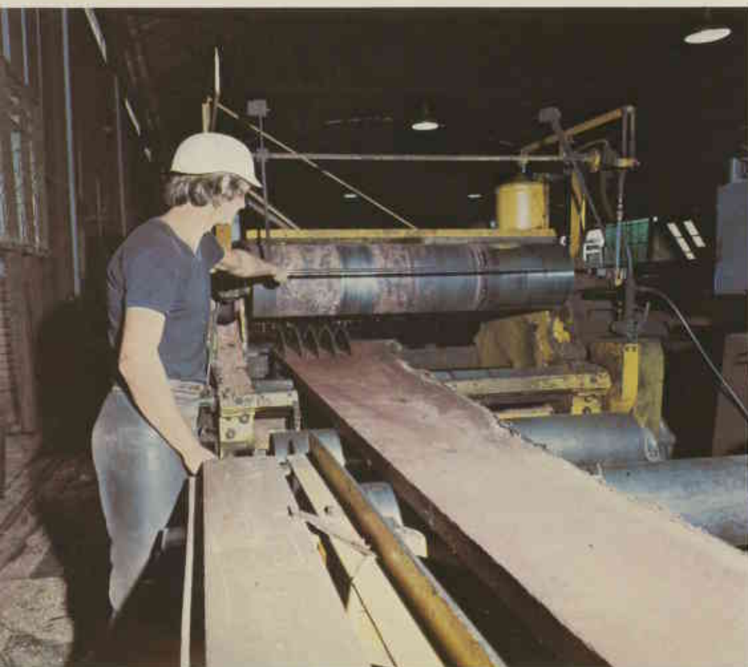
◀ Gang circular saws processing slabs into dimensioned scantling timber. The slabs for this unit come directly from the twin circular breakdown saws shown above.
