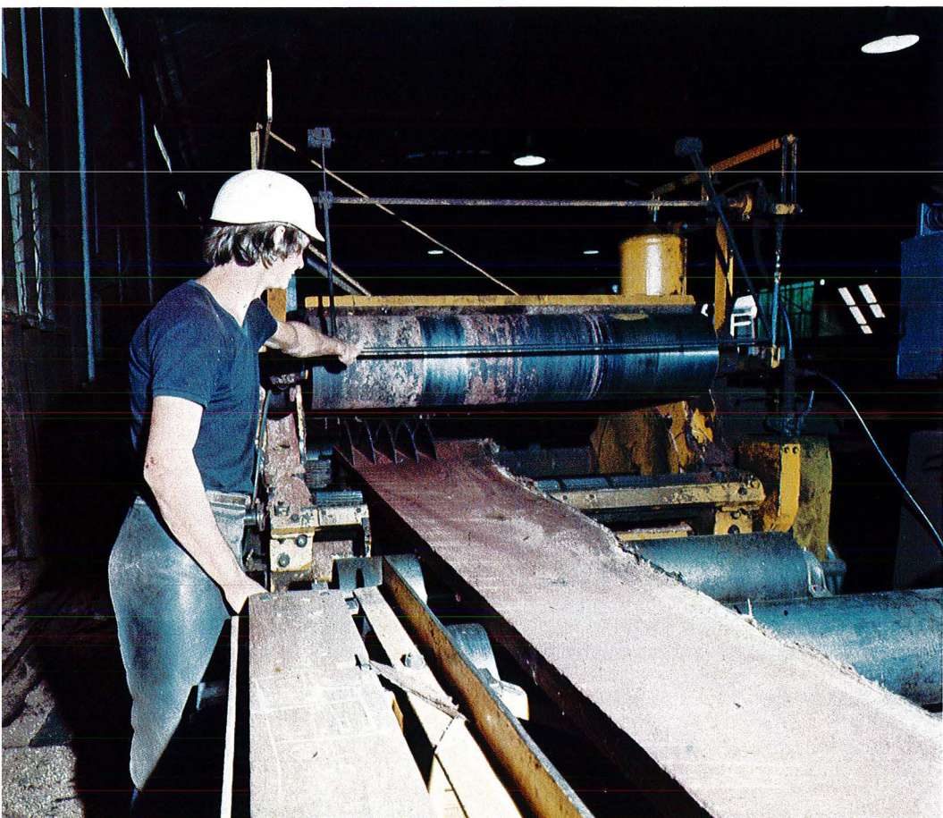
◀ Gang circular saws processing slabs into dimensioned scantling timber. The slabs for this unit come directly from the twin circular breakdown saws shown above.
