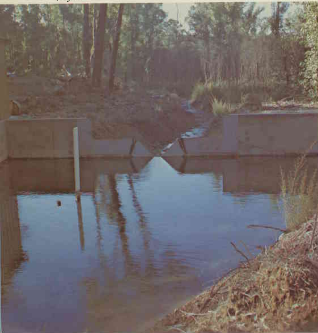
▼ Stream gauging station. By measuring rainfall, streamflow and stream salinity, a hydrological budget can be constructed for a catchment.
