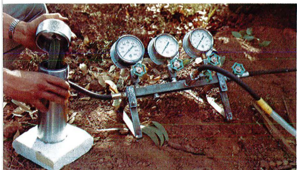
▼ Stomatal resistance meter estimates rate of leaf transpiration.
