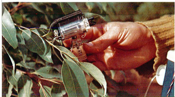
▼ Stomatal resistance meter estimates rate of leaf transpiration.
