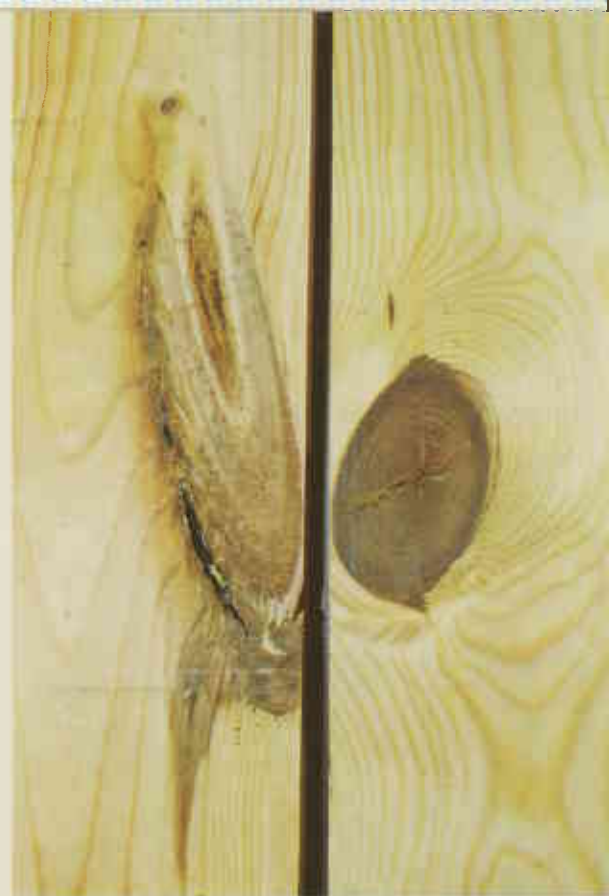
Pine boards degraded by large knots, ▲ one of the most serious defects of pine timber. Larger board 170 mm wide.
