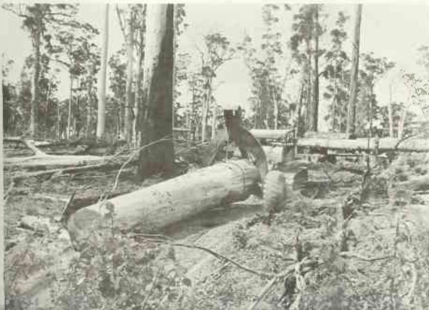
▼ Logging karri with a bulldozer and rubber-tyred arch in the late 1960s.
