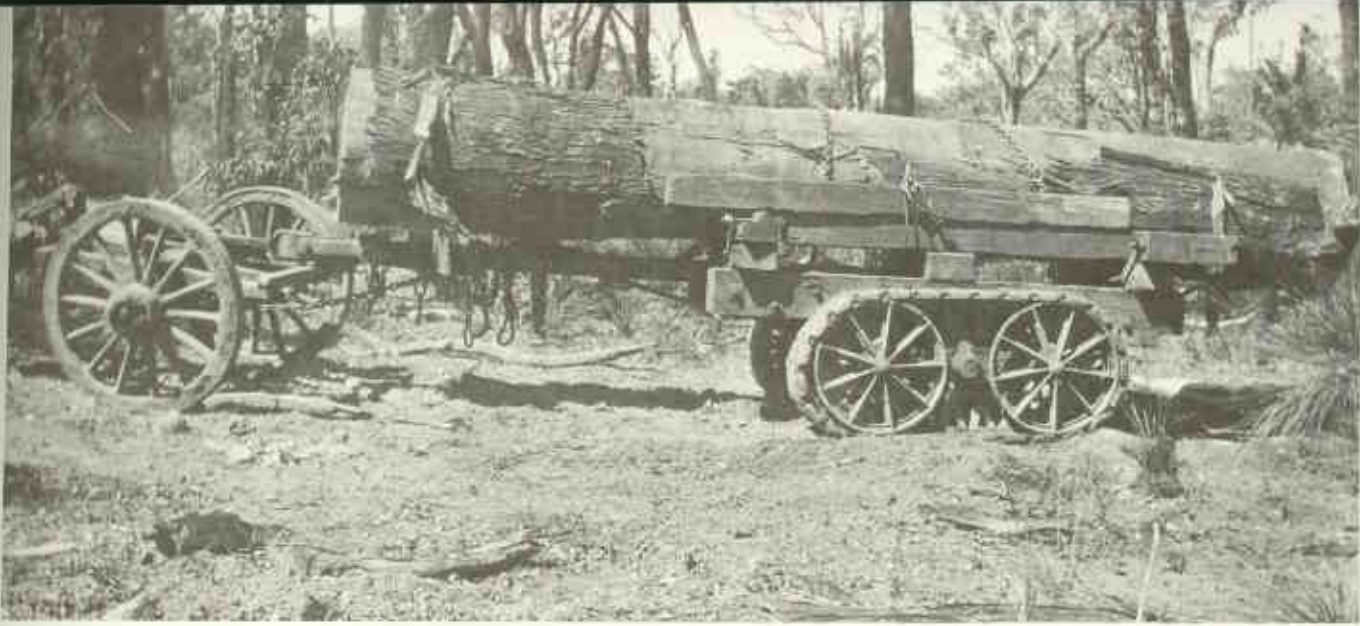
▲ Crawler-tractor drawn jinker. Note the tracked rear bogies.
