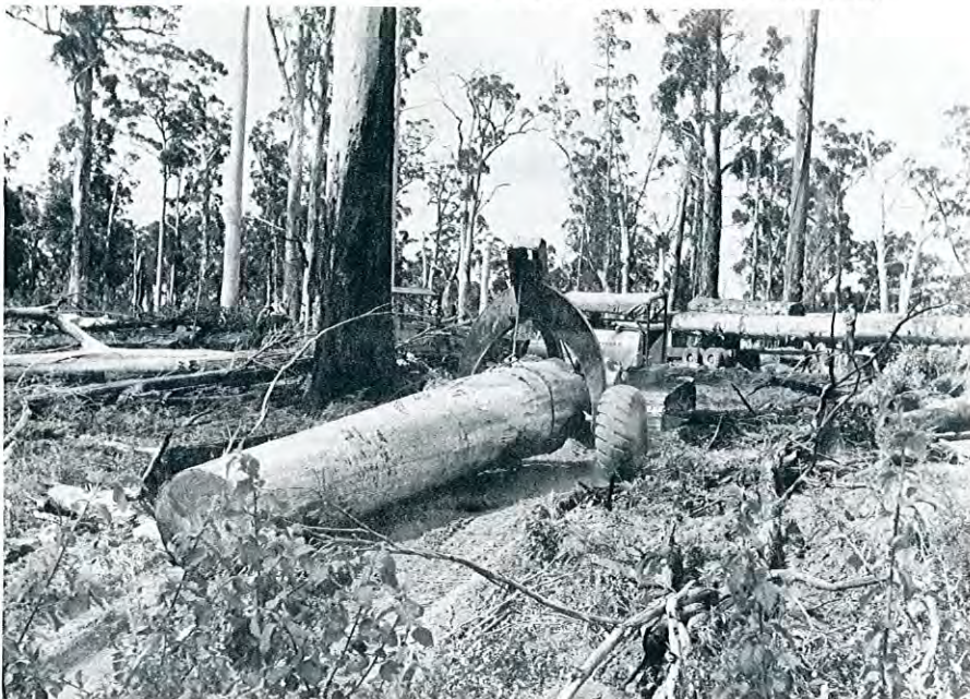
▼ Logging karri with a bulldozer and rubber-tyred arch in the late 1960s.
