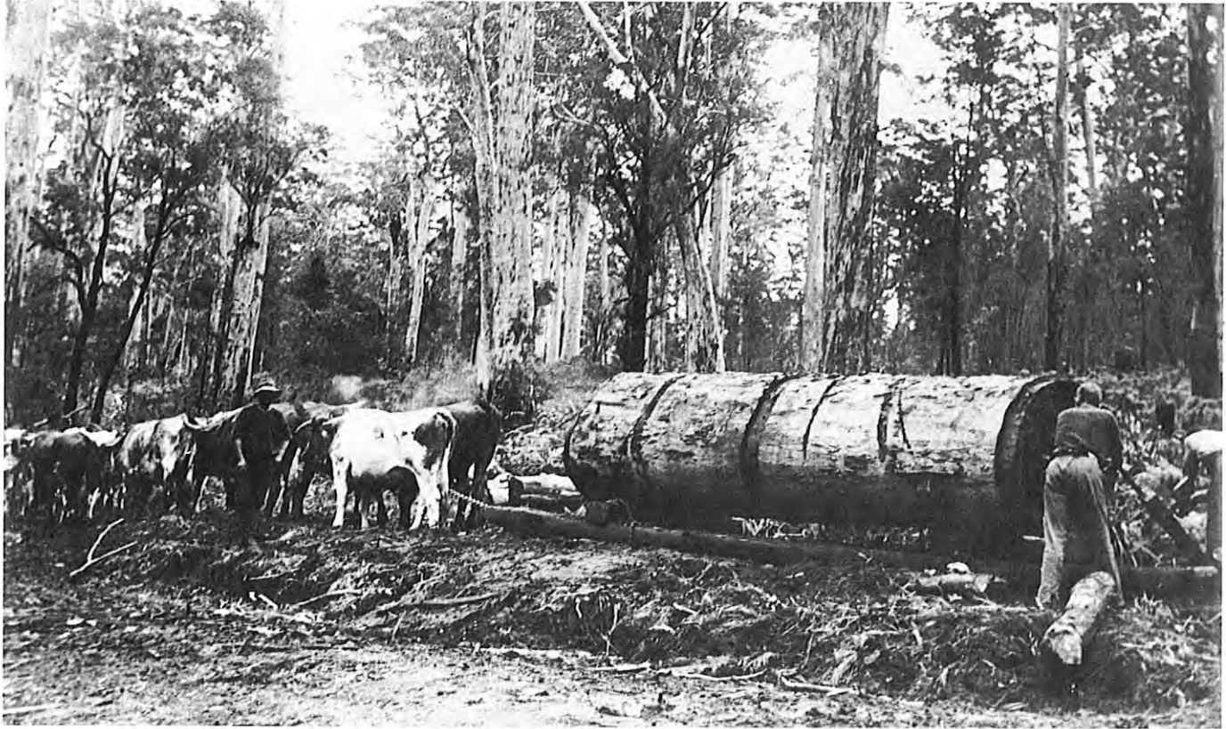
▲ One of a number of methods of snigging logs which were tried during the early days.
