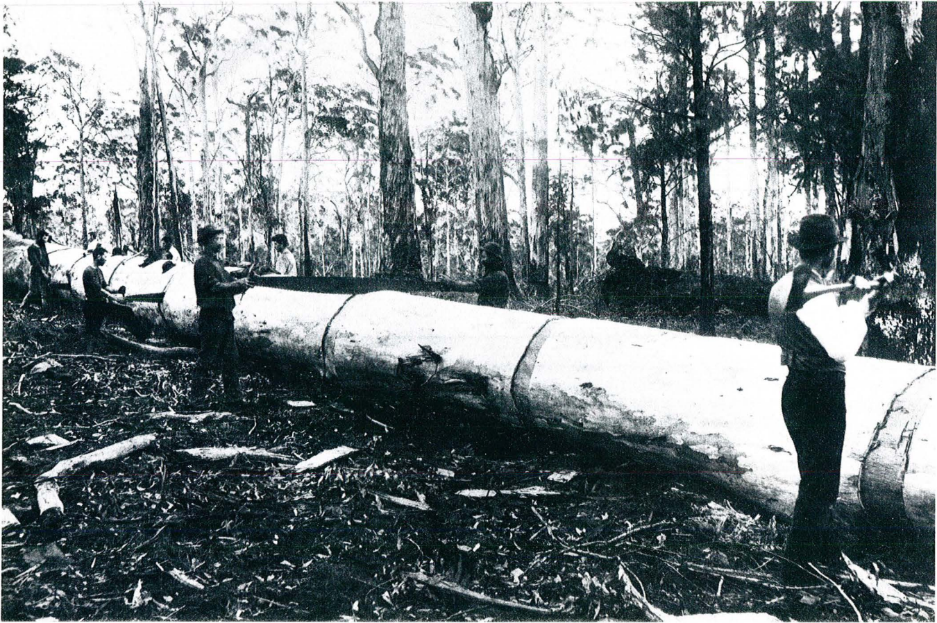
▲ Cross-cutting karri log (working up from the stump end) ready for snigging to log landing.
