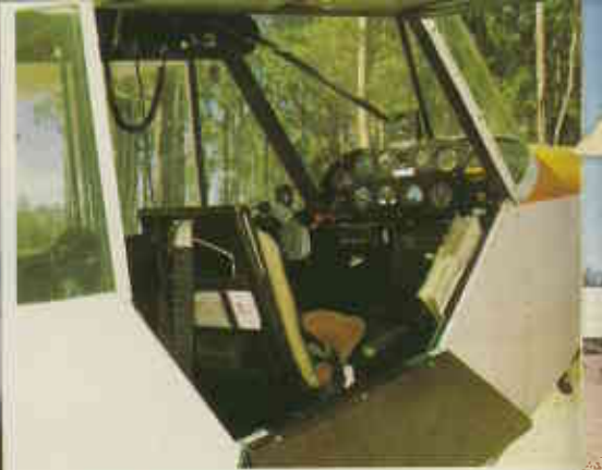
▲ Inside the Super Cub. The tandem seating arrangement is especially suited to surveillance work, as 180° viewing is available without tilting the aircraft. (Les Harman)
