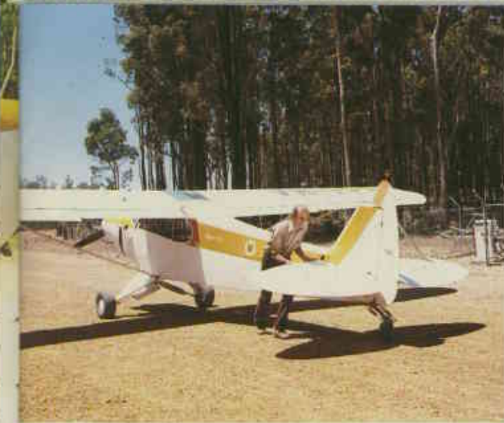
▲ Made from stressed metal and fabric coated with a plastic Dacron finish, the Super Cub is strong, but light enough for one person to wheel in and out of the hangar. Here John Woodward wheels the aircraft out on to the taxi-way. (Les Harman)
