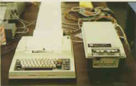
▲ The terminal interface (left) is operated by the navigator who types in co-ordinates of the desired flight line. The tape-deck records plotting co-ordinates for later mapping and matching with photographs.
