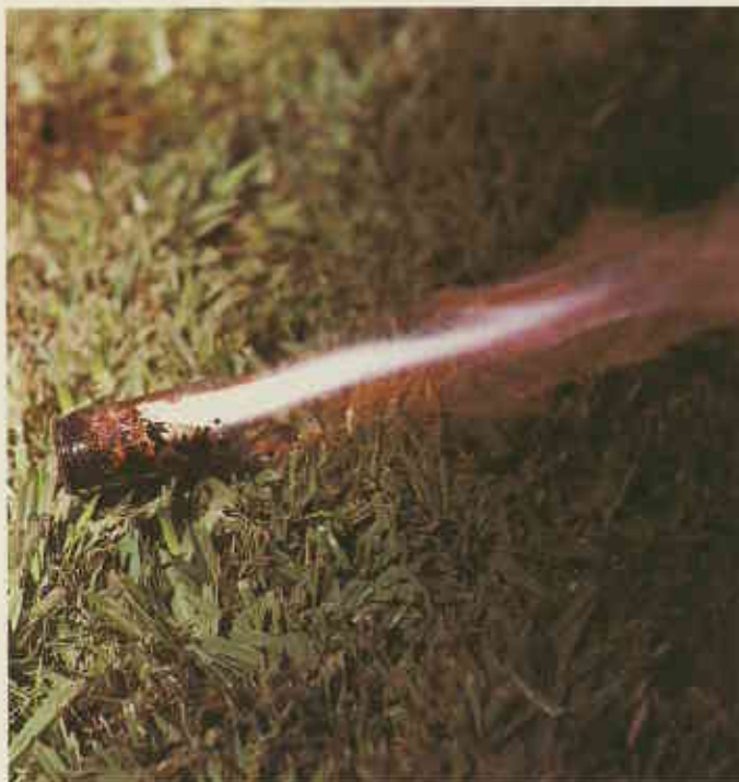
▲ The ignition capsule, an incendiary "bomb", has gone through many stages of development, including the current one of potassium permanganate crystals held in a plastic cylinder. It is shown here igniting 30 seconds after having been injected or "primed" with a catalyst. (G. van Didden)
