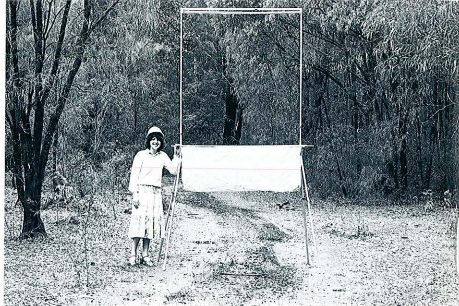
Bat trap. Bats fly into two sets of closely spaced nylon fishing lines strung on an aluminium frame. They fall into the sack below, crawl up underneath an overhang and settle down to sleep awaiting the arrival of the trapper in the morning. (T. Leftwich)
