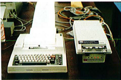
▲ The terminal interface (left) is operated by the navigator who types in co-ordinates of the desired flight line. The tape-deck records plotting co-ordinates for later mapping and matching with photographs.
