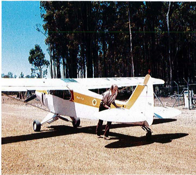
▲ Made from stressed metal and fabric coated with a plastic Dacron finish, the Super Cub is strong, but light enough for one person to wheel in and out of the hangar. Here John Woodward wheels the aircraft out on to the taxi-way. (Les Harman)
