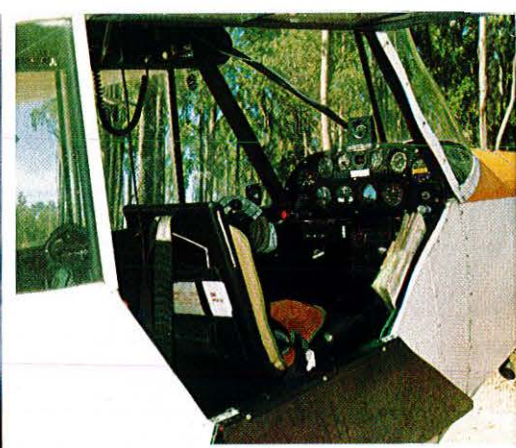
▲ Inside the Super Cub. The tandem seating arrangement is especially suited to surveillance work, as 180° viewing is available without tilting the aircraft. (Les Harman)
