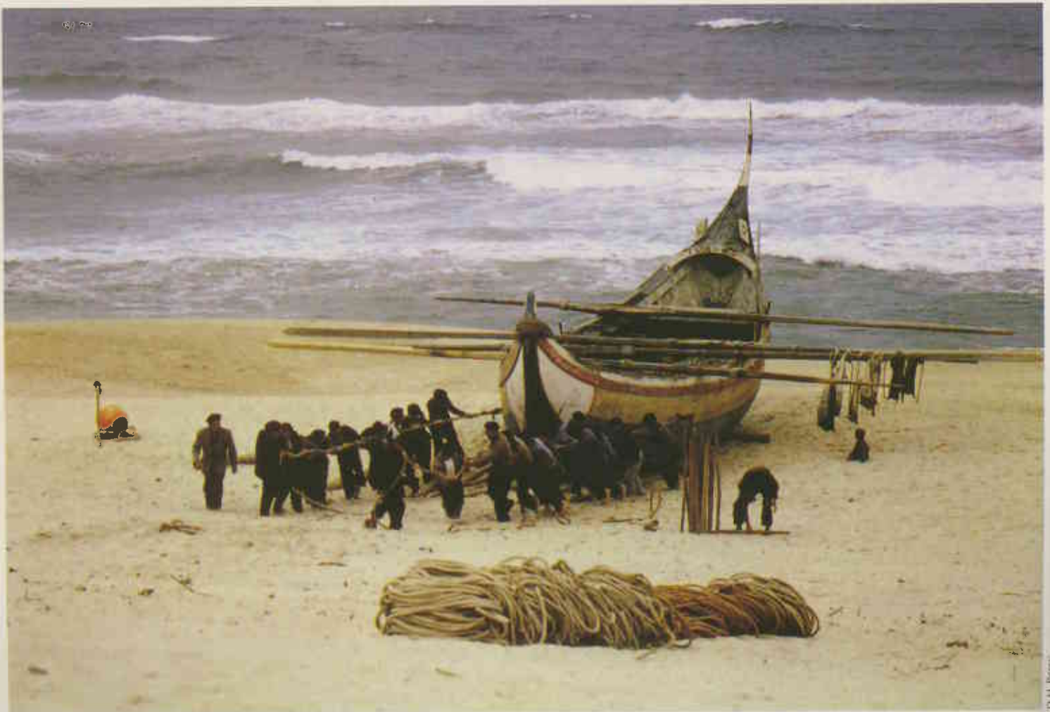
The Portuguese have used maritime or pinaster pine in ship building for centuries. Here the villagers haul the longboat in after a fishing expedition. The hull and oars are all made of pinaster.
