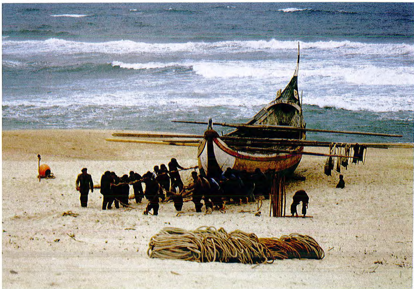
The Portuguese have used maritime or pinaster pine in ship building for centuries. Here the villagers haul the longboat in after a fishing expedition. The hull and oars are all made of pinaster.
