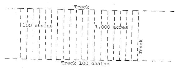
In an area of 1,000 acres, say 100 chains by 100 chains, would require 20 lanes 100 chains long. That is 25 miles of lanes plus 200 chains travelling between lanes.
