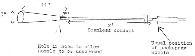
The nezzle has an extra large lever to facilitate movement when hot. The normal packspray nozzle aperture tends to be too large and the unit is more efficient if the jet is slightly burred around the edges.
