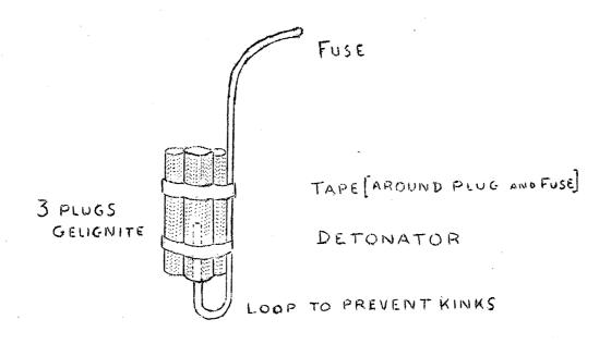
Three plugs of Gelegnite are then taped together with Durex tape and a convenient length of safety fuse with detonater inserted into one plug.
