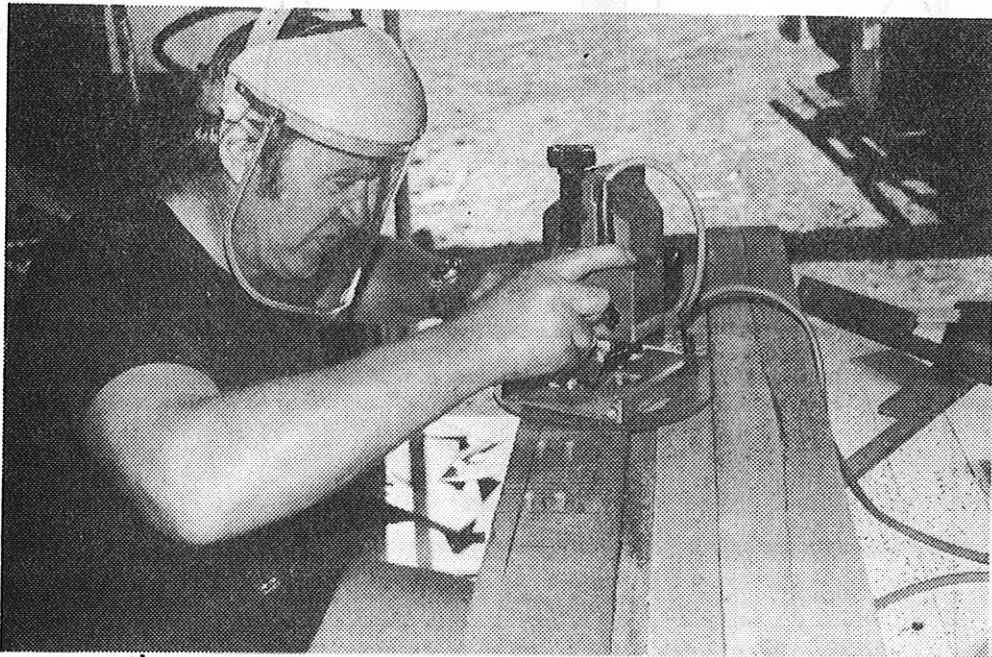
Router in use with straight vertical jig
