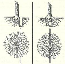
Tunnel beneath root systems. Drawings at left show trenching that would probably kill the tree. Drawings at right show how tunnelling under the tree will preserve many of the important, feeder roots.
