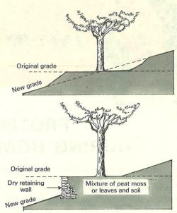
Terracing with a retaining wall protects a tree from a lowered grade.
