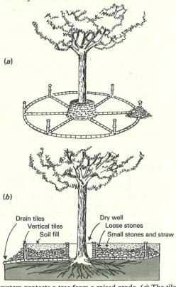
A tile system protects a tree from a raised grade. (a) The tile is laid out on the original grade, leading from a dry well around the tree trunk. (b) The tile system is covered with small stones to allow air to circulate over the root area.
