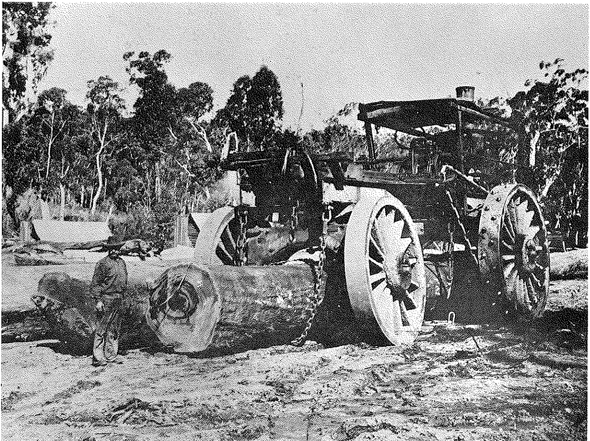
Steam Power: The "Harry Stevens" mechanical log hauler—reputedly the first of its kind in Australia. It had 3.35 m rear wheels chain-driven by a vertical-boiler steam engine.
