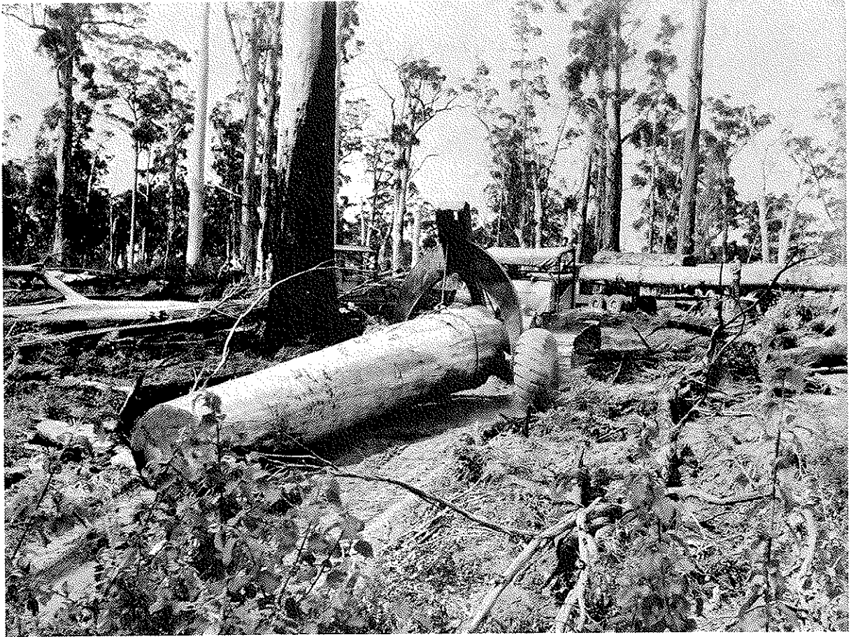
Rubber-tyred logging arch in the karri forest in the 1960s.
