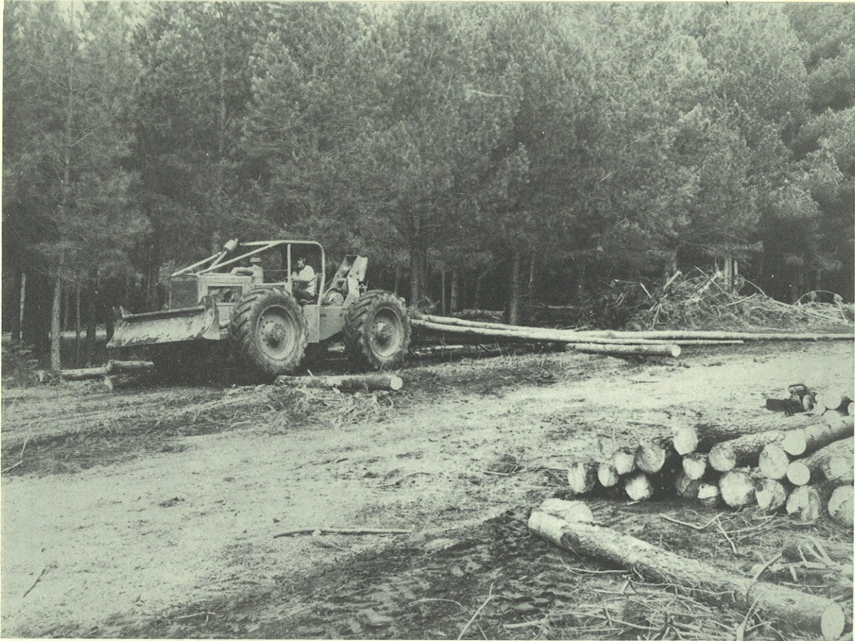
BELOW: Rubber-tyred logging arch in the karri forest in the 1960s.
