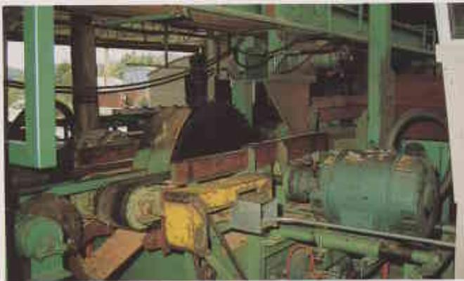
The twin-bladed breaking down saw. (Top)
