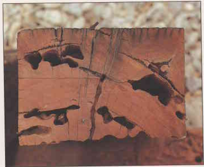
Mastotermes are virtually unstoppable. An attack on a jarrah sleeper (above) and on a karri sleeper which had been treated with dieldrin and creosote (below).
