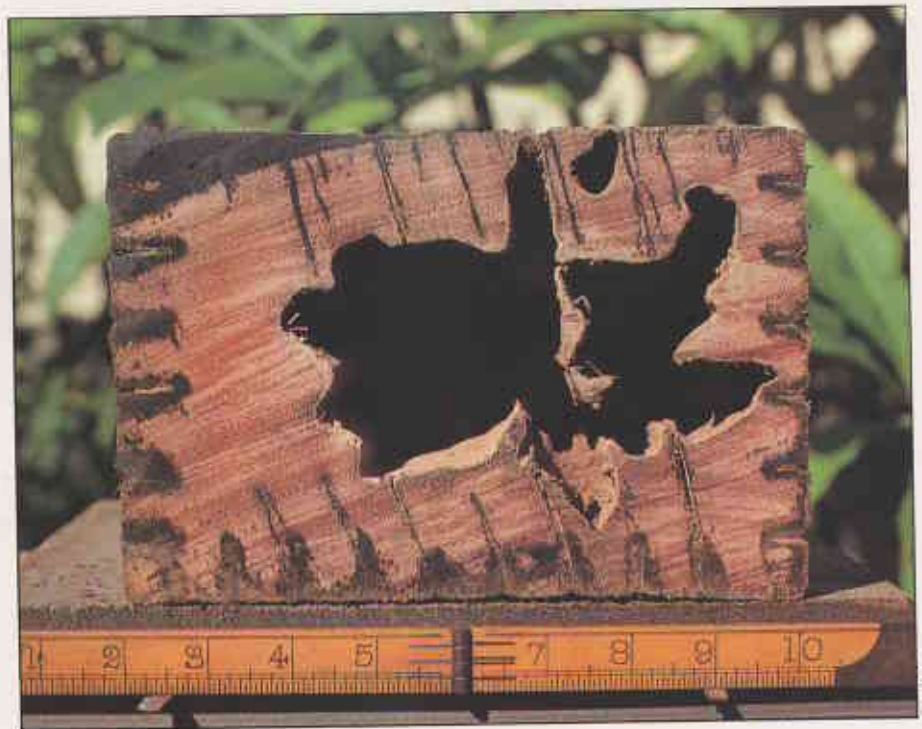
Mastotermes are virtually unstoppable. An attack on a jarrah sleeper (above) and on a karri sleeper which had been treated with dieldrin and creosote (below).
