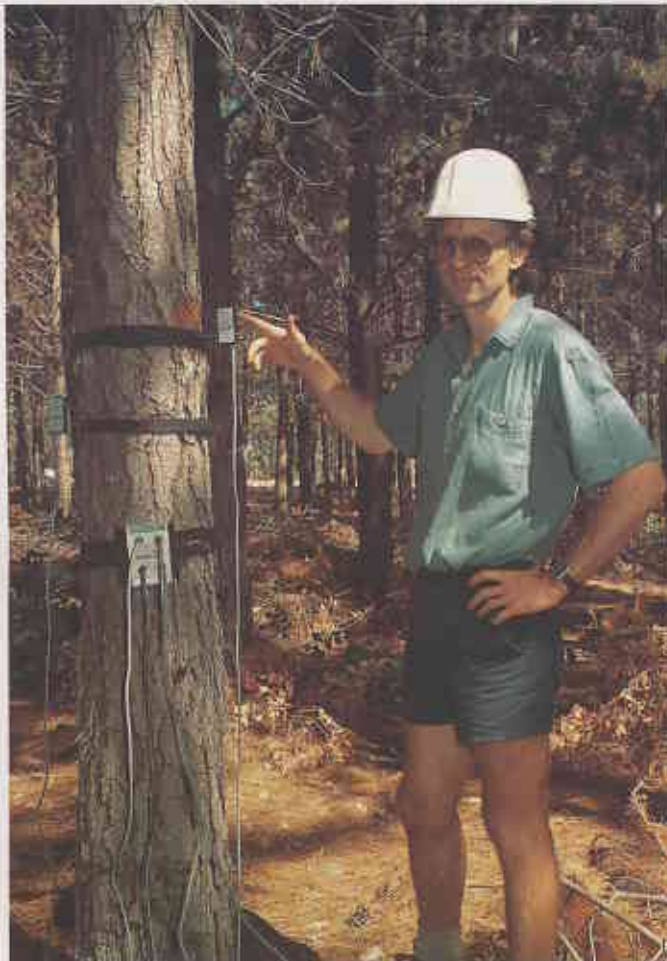
Left: Joe Kinal points to a sap-flow meter inserted into a radiata pine.
