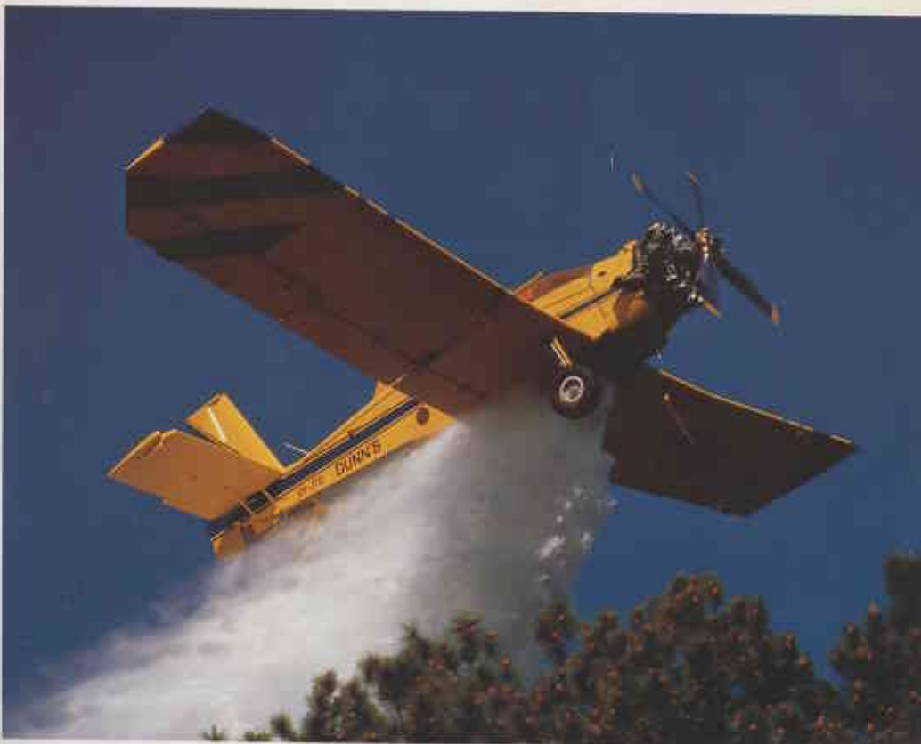
An aerial water bomber releases its load as it flies low over the treetops.
