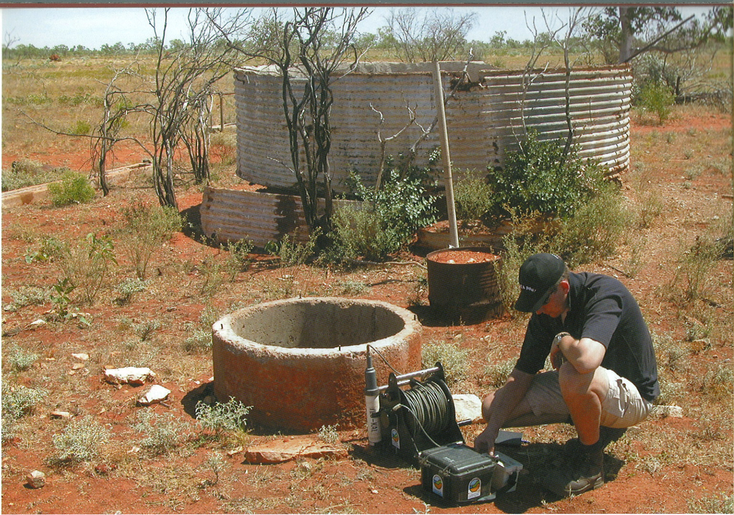
Above CALM technical officer Jim Cocking measures water chemistry at Nimingarra Well on Muccan Station. Photo – Mike Scanlon/CALM
