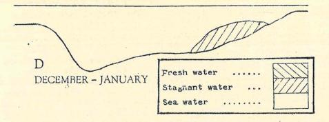
Between B and C the stagnant zone is shifted to and fro by water-level changes brought about by barometric pressure - not rainfall discharge. When the water level is low this zone moves downstream under the influence of water leaving the river; as the water level rises it is pushed back by marine water entering as in figure B.
