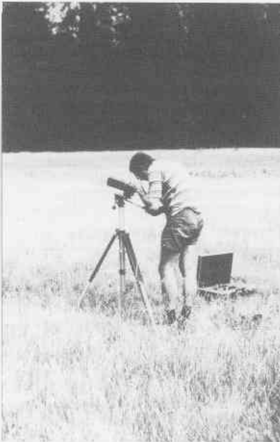
x 40 Questar telescope, Yosemite National Park. Telescope is focused on rock climbers on a major rock wall almost one kilometre away. When used with a loud hailer, the telescope can be a great asset during big wall rescues.
