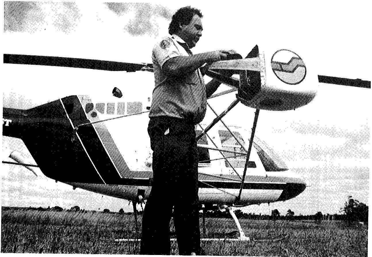
Figure 9 Camera pod with rear housing removed.
