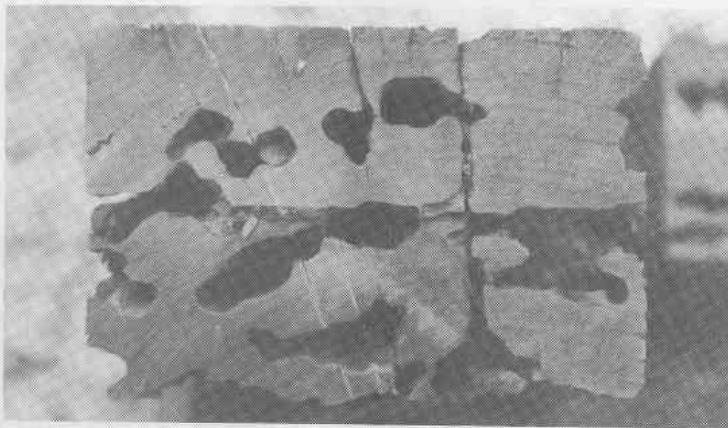
FIGURE 3: An untreated jarrah sleeper, showing galleries being excavated by Mastotermes darwiniensis .
