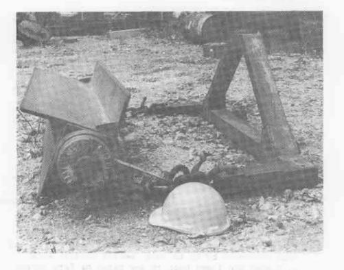
FIGURE 1: Scrub roller used for crushing thinning slash
