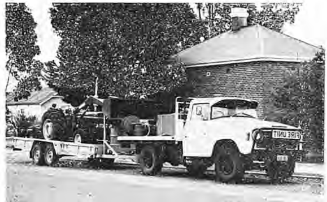
Mobile fire fighting unit with trailer-borne tractor.
