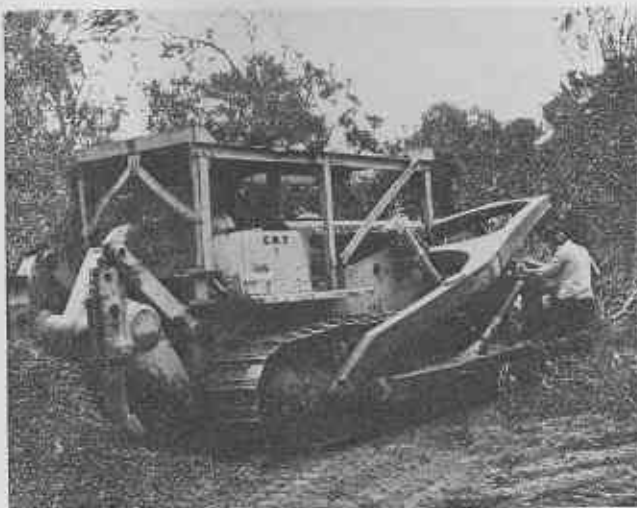
Clearing timber from the dozer during fire break maintenance.
