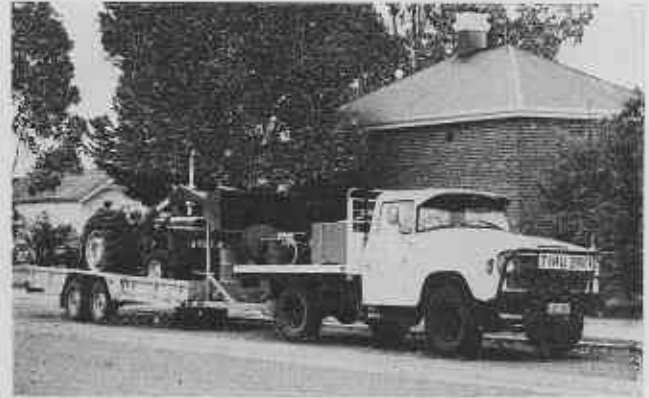
Mobile fire fighting unit with trailer-borne tractor.
