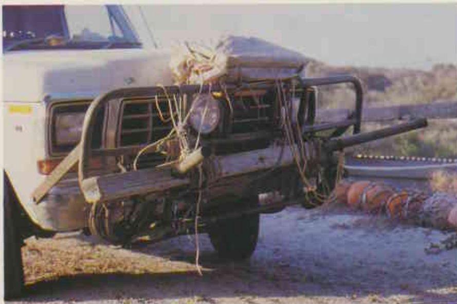
▲ The cannon net loaded and ready to fire in early prototype. (Photo G.Pearson.)
