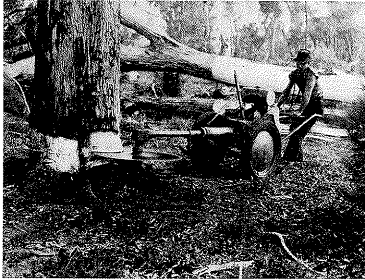
Falling trees with a modern power-operated circular saw.
