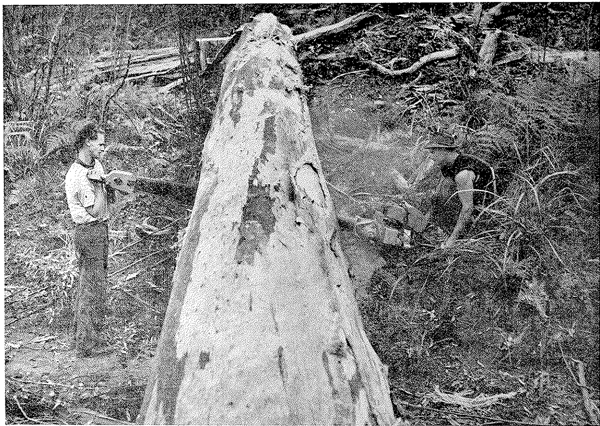
Plate 3.—Cross-cutting a large Karri log prior to snigging to the landing.
