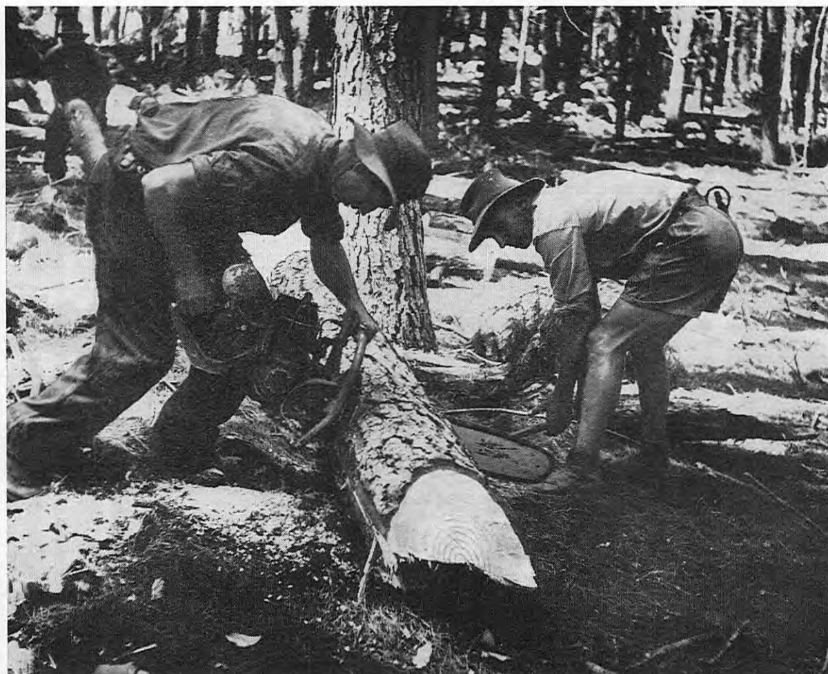
Cross cutting Pinus radiata into "peeler logs" using a power chain saw at Mundaring Plantation
