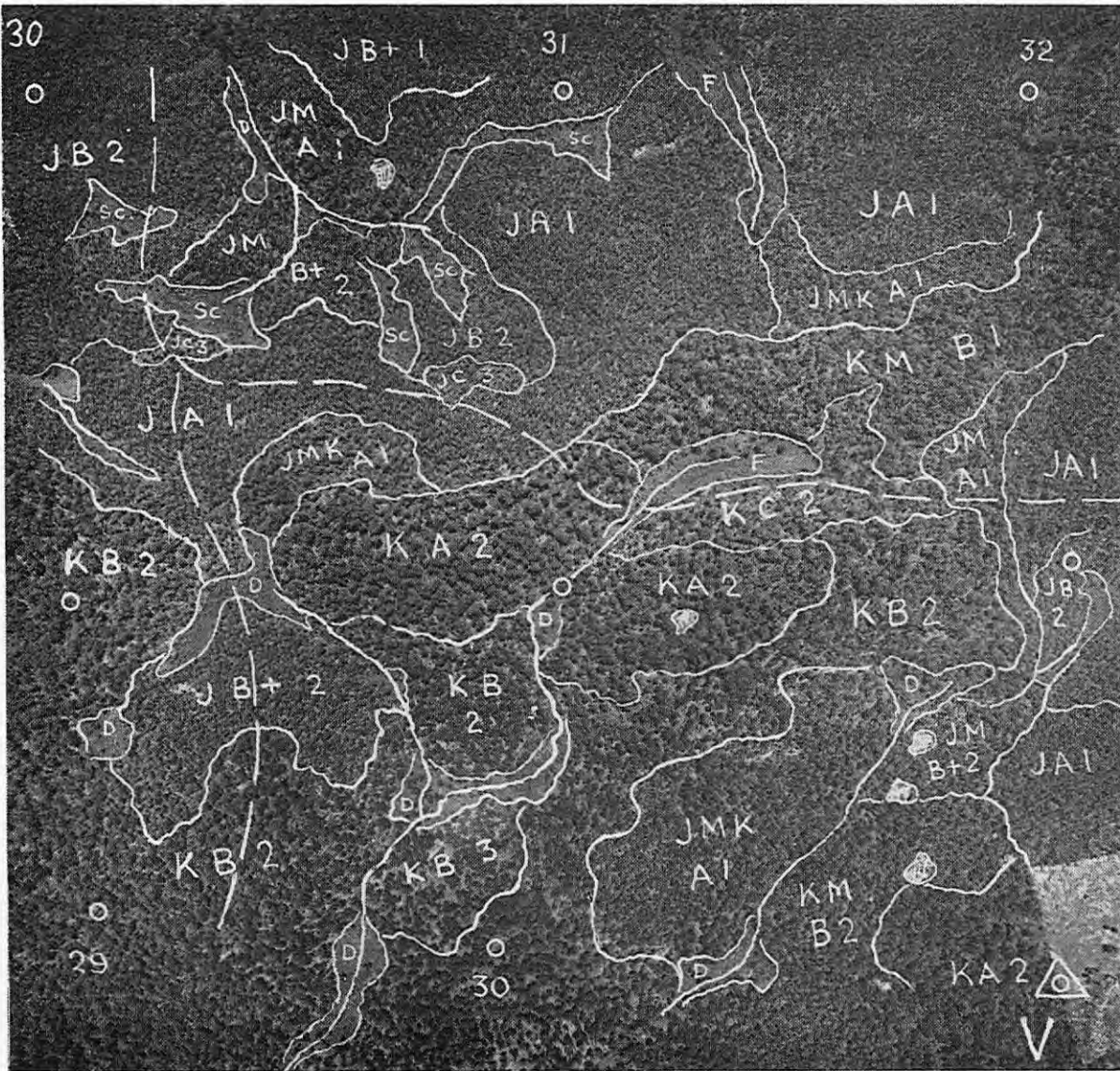
Forest Mapping from air photographs. A marked air photo showing interpretation of karri and jarrah forest in the far south
