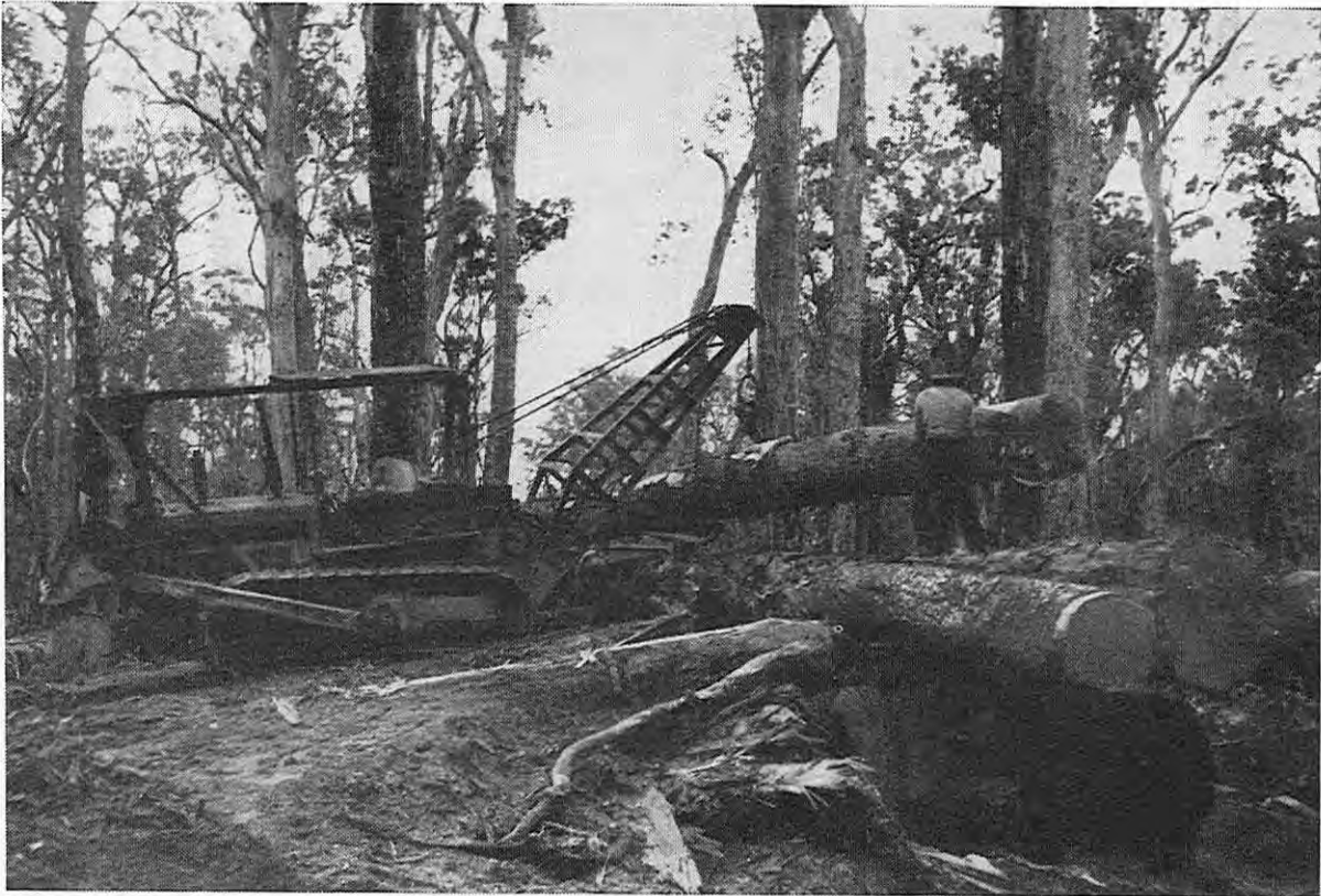
Loading jarrah logs with a tractor mounted crane in a mixed jarrah-karri forest
