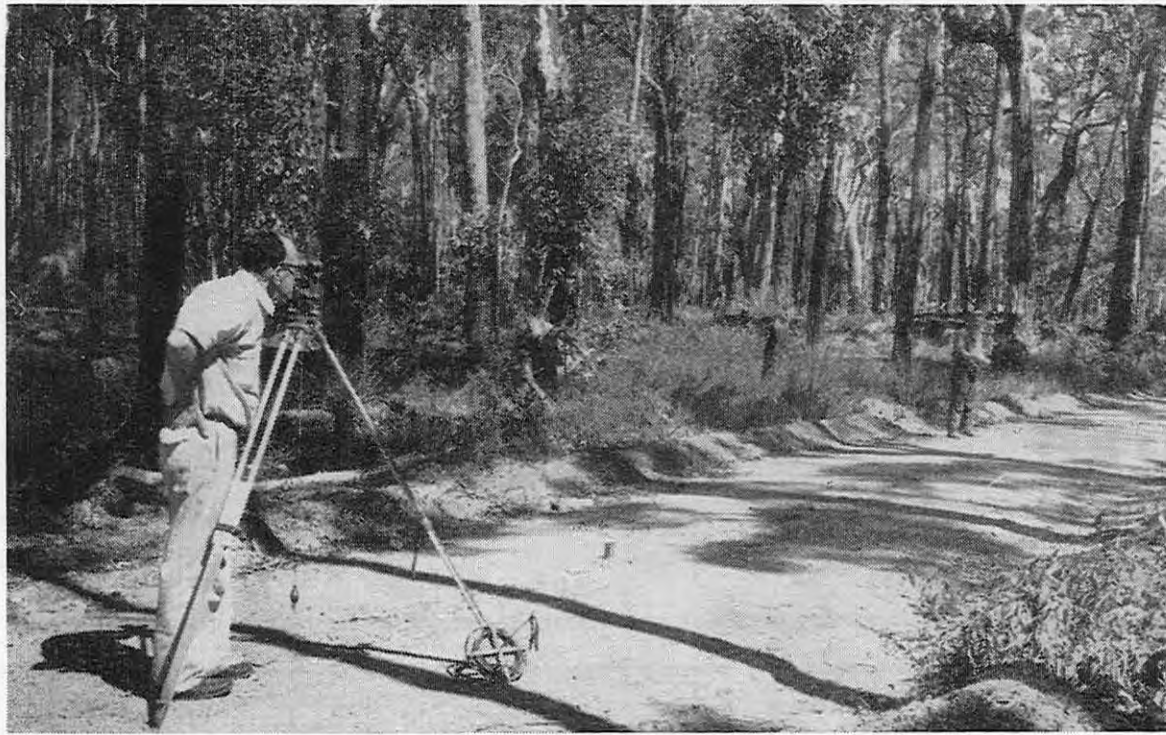
Theodolite surveying for mapping control
