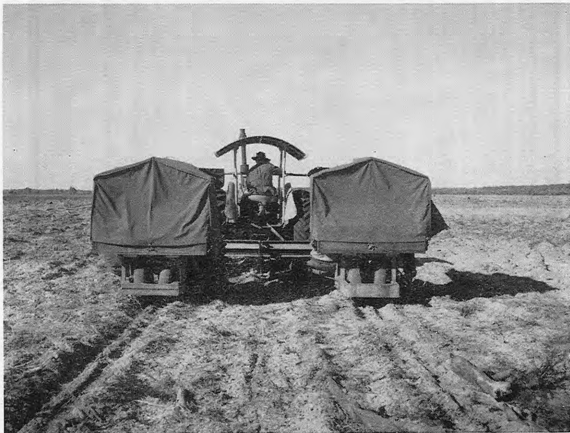
Pine Establishment. A "Lowther" dual operation planting machine in action
