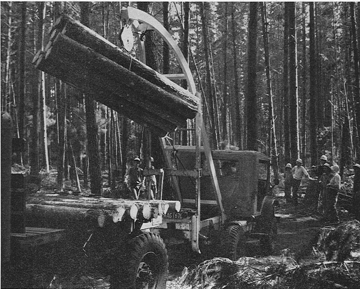
Forest trainees observe the operation of a jib-crane loading small pine logs in the Grimwade plantation.
