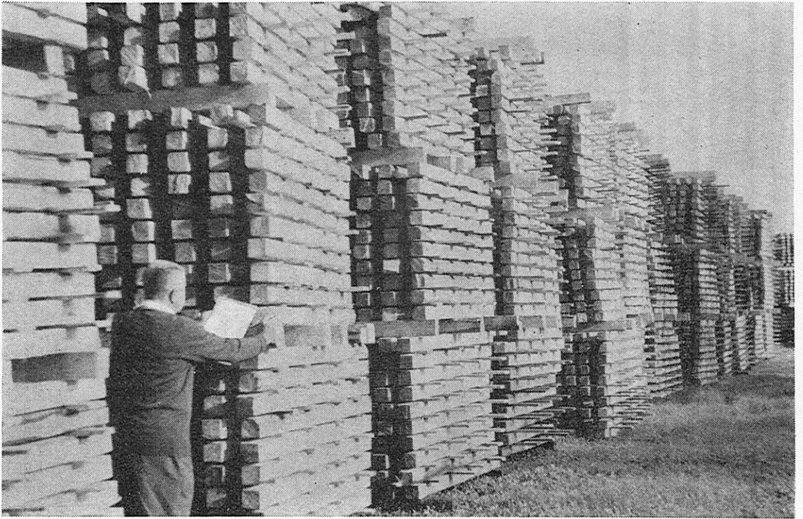
To supplement supplies of case material, these pine flitches or baulks, are cut at a mill near Busselton and air-dried before railing to the case factory in Perth.
