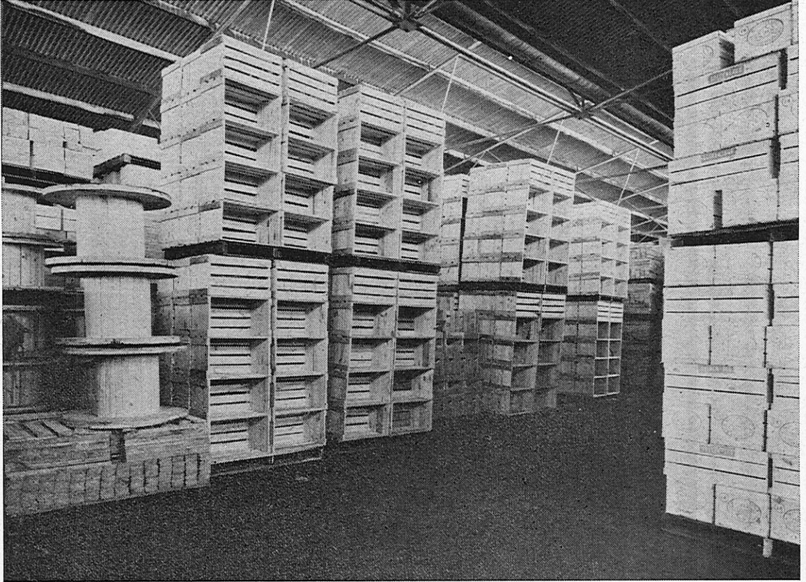
Some of the end products from pine case logs and flitches. As well as cable reels, the photograph shows various cases and crates for the packaging of such produce as eggs (export), fruit, vegetables, fish and mineral waters.
