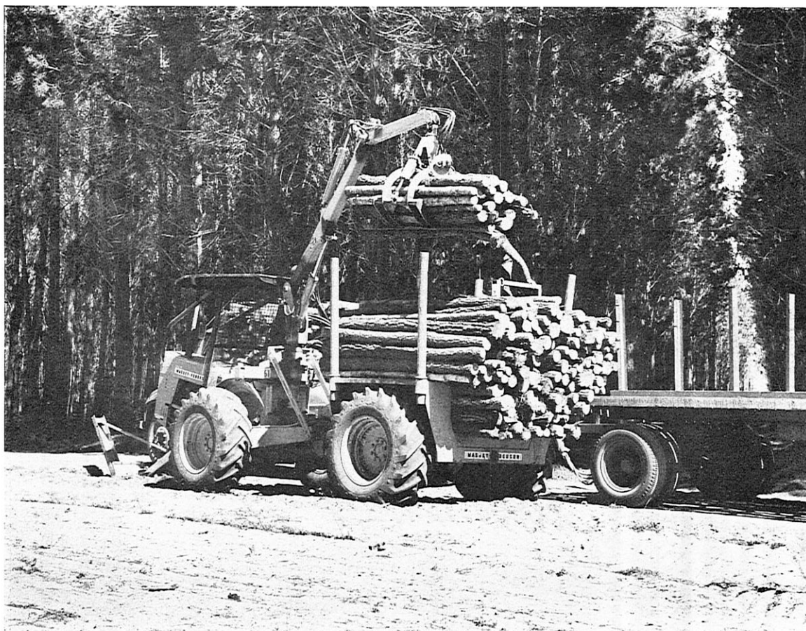
“ A Massey-Ferguson 2200 Treever operating in Gngalara plantation ( P. pinaster ). Operated by one man, the machine handles in a given time a greater volume of logs from first thinnings than the previous system of two and sometimes three crane trucks with their higher man-power requirements.”
