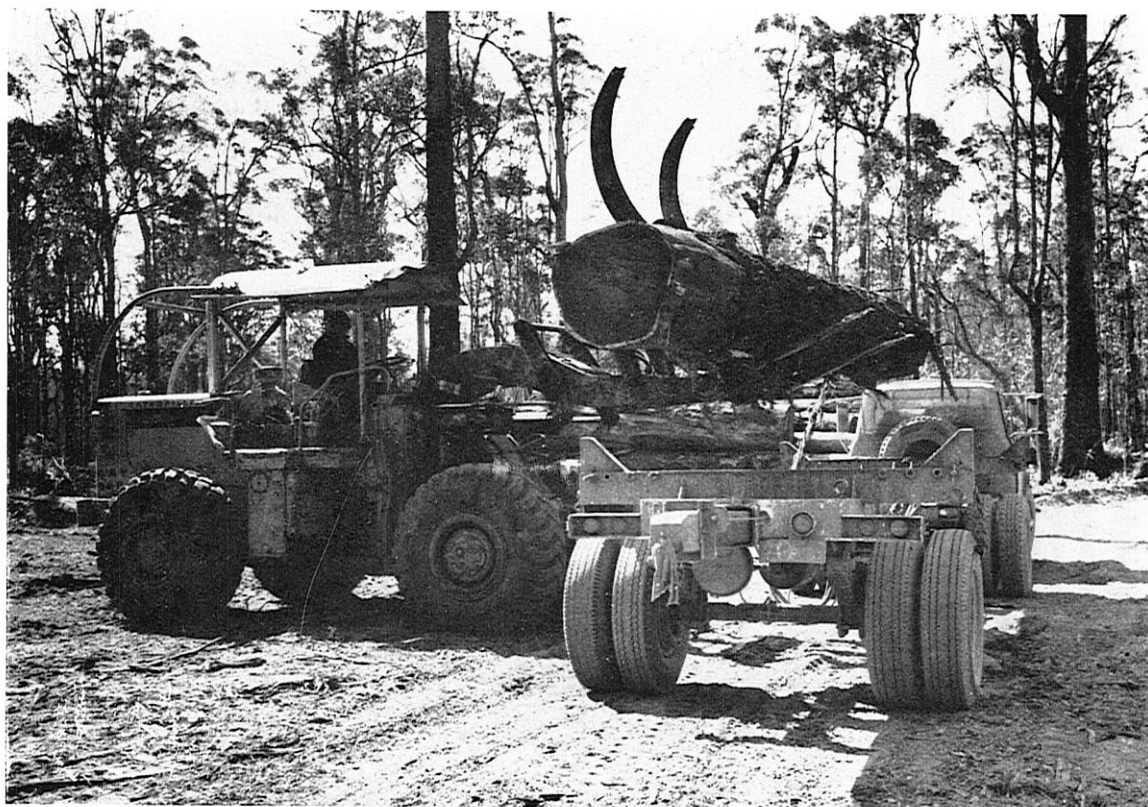
“ Rubber-tyred logging units have greatly increased in popularity in recent years, particularly in the jarrah forest where logs are smaller than in the karri forest. The photograph shows a Caterpillar 966B loading a jarrah log onto the jinker of a waiting log truck.”
