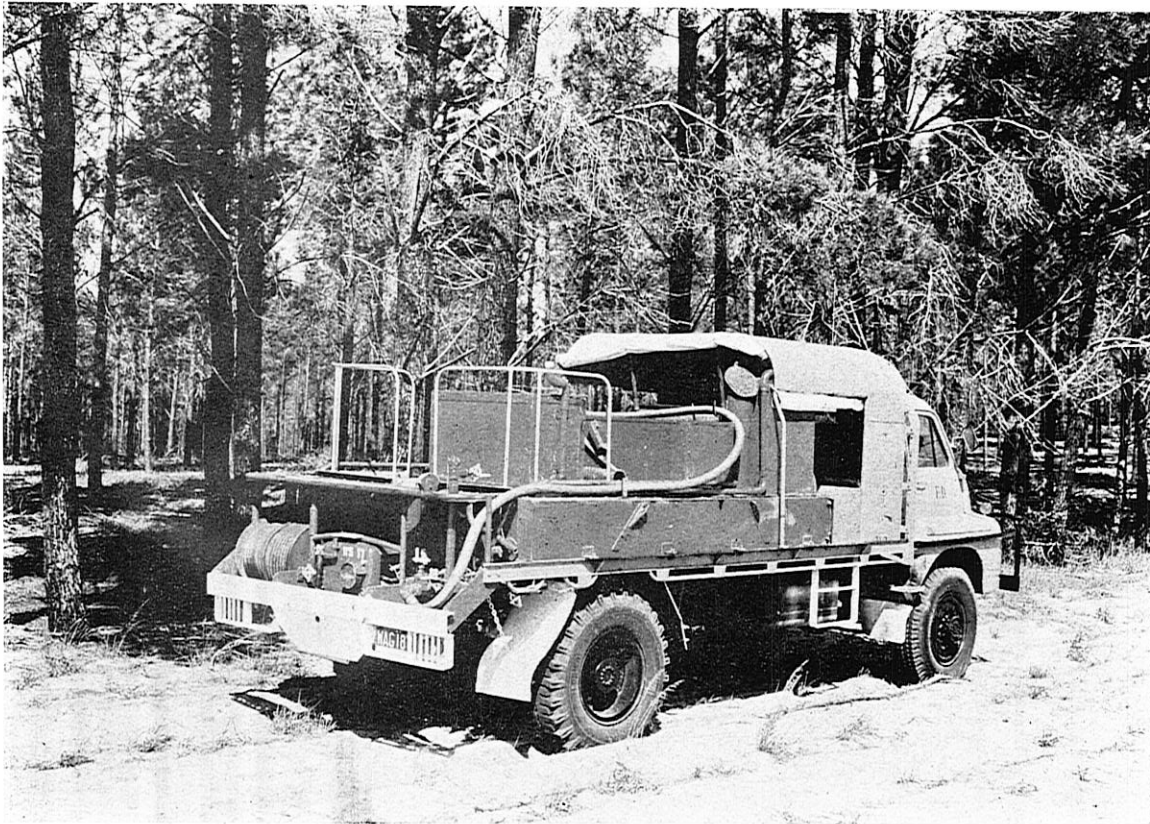
"The new 'heavy duty outfit' or tanker unit is designed as a dual purpose fire fighting unit and personnel carrier. The unit incorporates a 600 gallon capacity 'flat' tank, the latest type high pressure pumper, crew seating (under shelter) behind the cab and 4 wheel drive."
