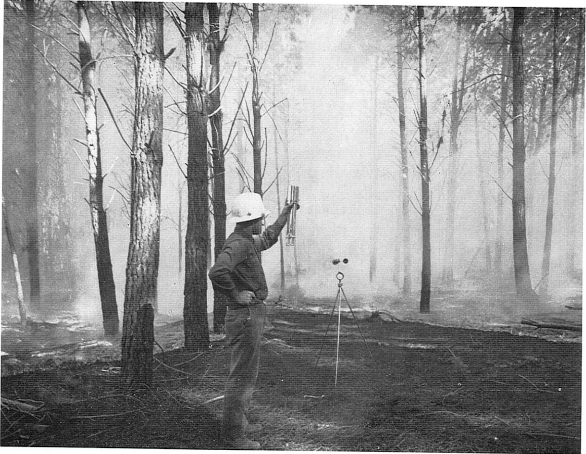
A careful record of prevailing weather conditions is required when experimental fires are lit in pine plantations. Here a fire research officer takes measurements of temperature, relative humidity and wind speed during burning trials in a stand of Pinus pinaster .
