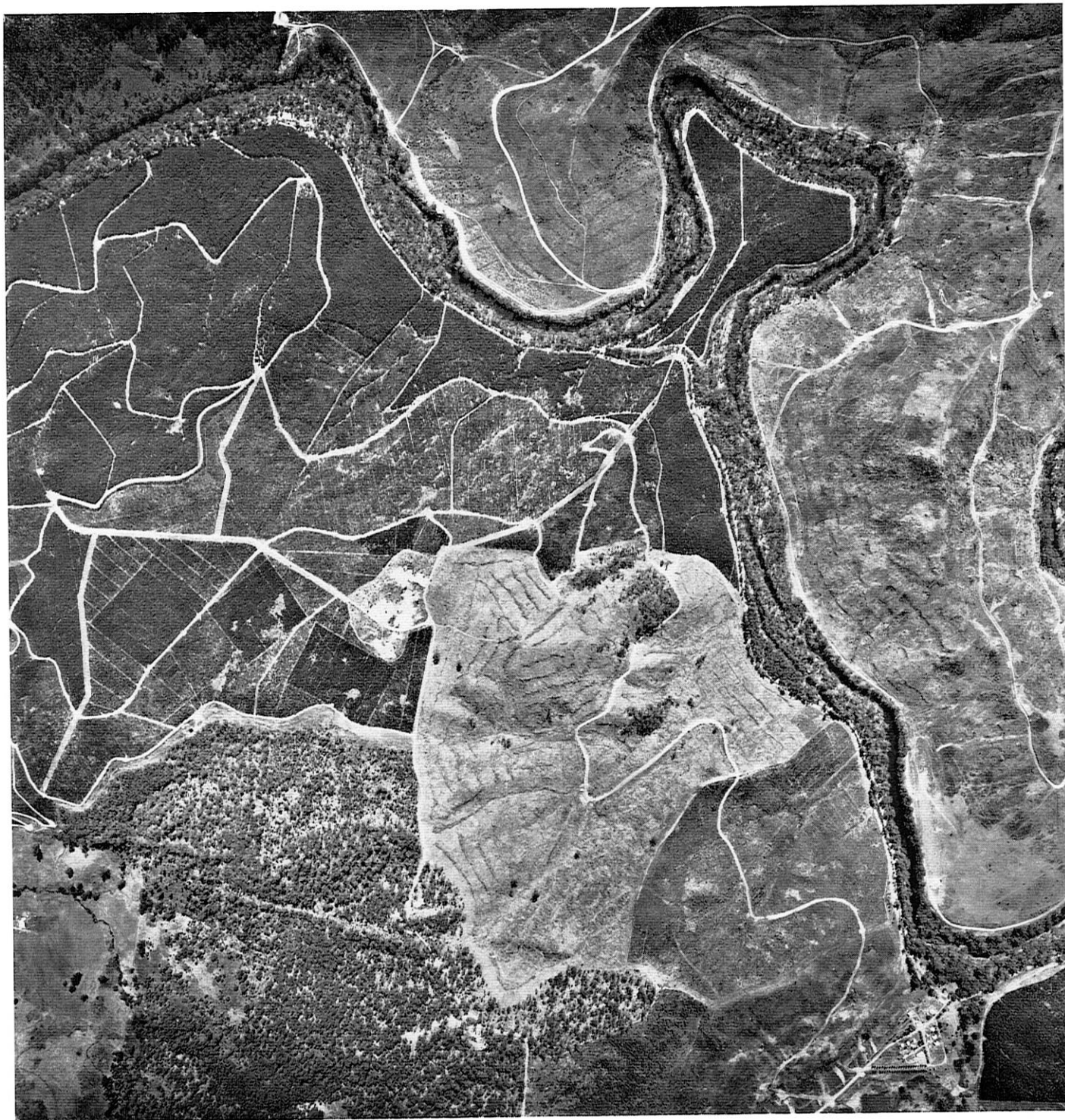
An aerial photograph of Pinus radiata at Lewana plantation, near Nannup. The photograph was taken with a 6-inch (15 cm.) lens from a flying height of 7,920 feet (2,414 m.) in April, 1969.
