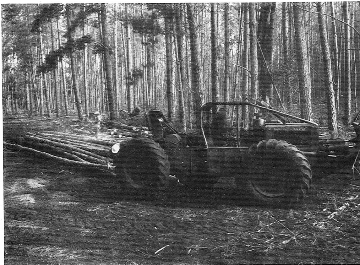
A Timberjack hauls long-length logs of 30 year-old radiata pine in Grimwade plantation (1971).
