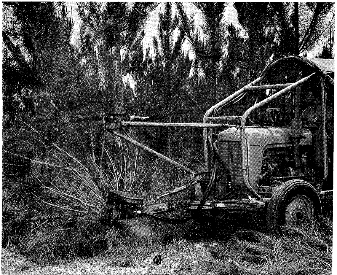
Tractor mounted circular saw which won an Award for its designer, Plant Inspector J. Reynolds, in 1974-75.
