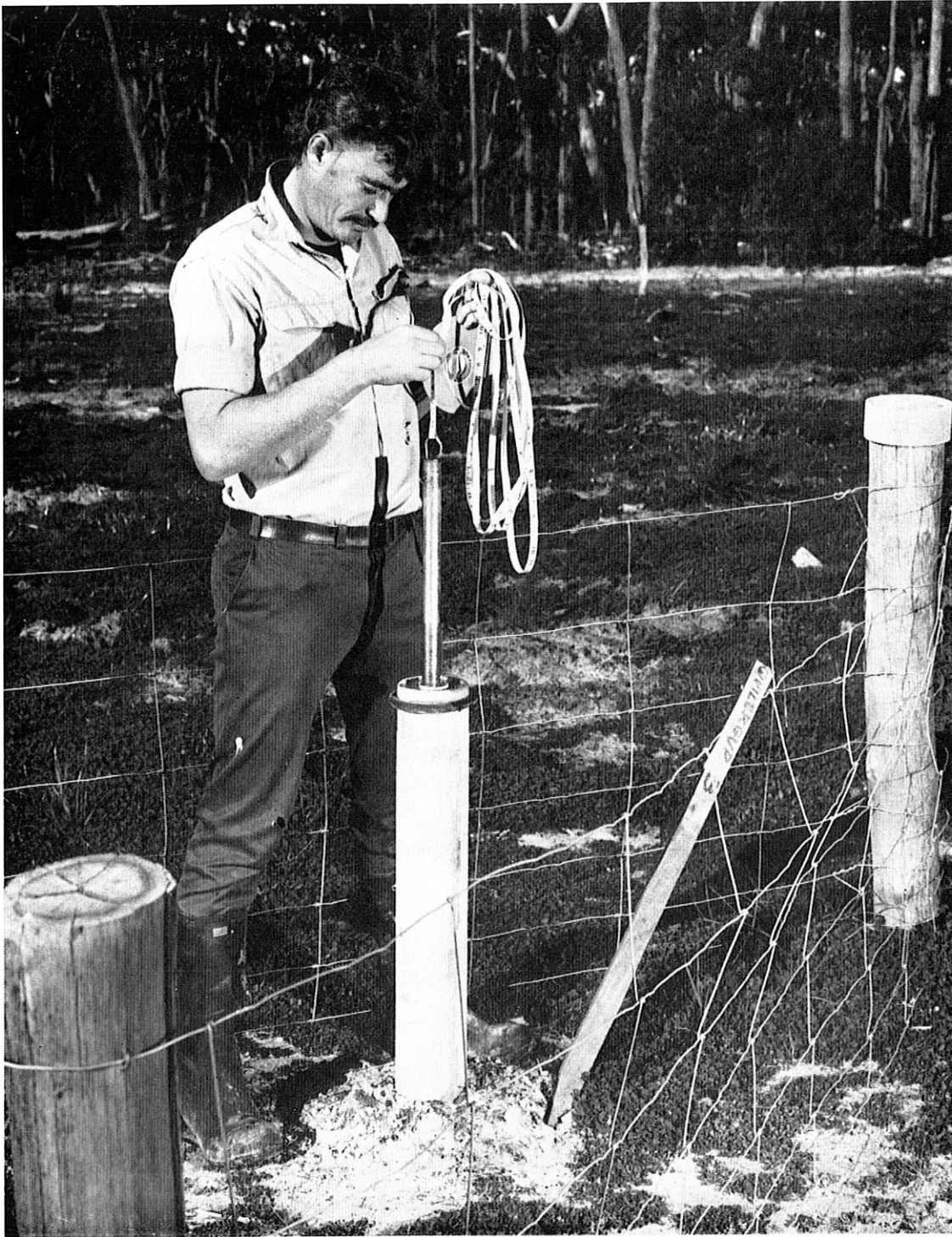
Bore-hole water sampling in the Jarrahwood area.
