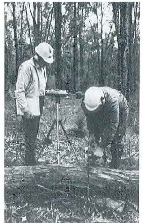
Safety Officer Tom Wood conducts a test of noise levels during chainsaw use.
