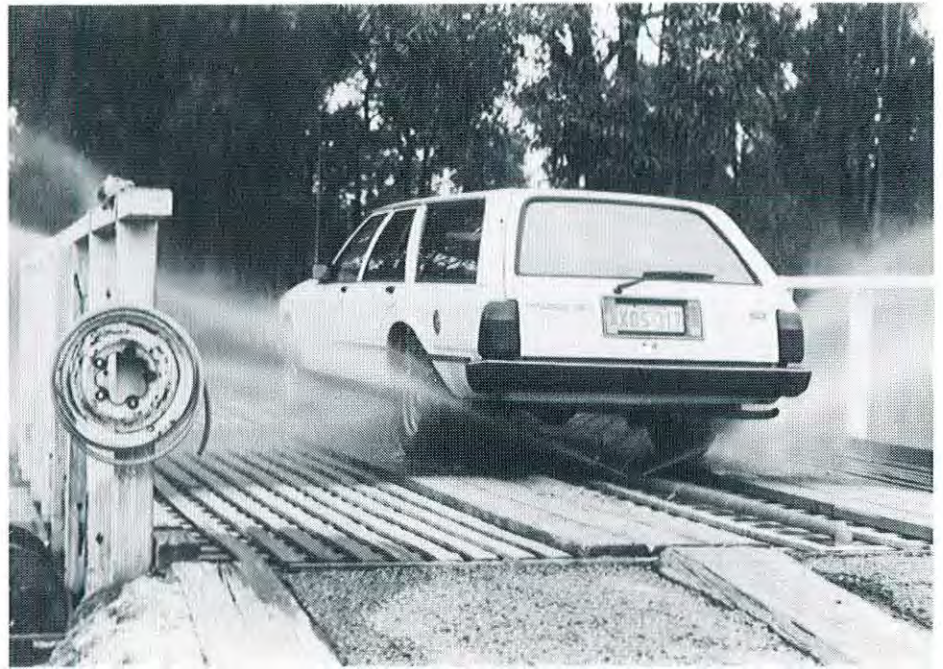
Wash down stations are still used throughout the forests as a means of containing the spread of the cinnamomi fungus by vehicles.
