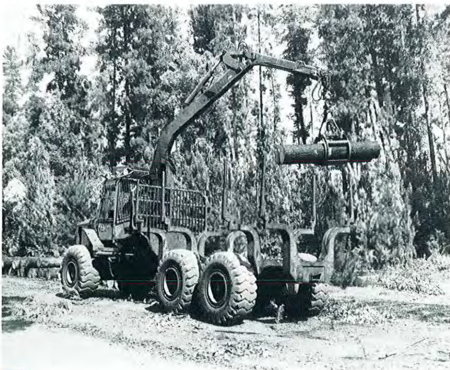
One of the Kockam Forwarders used to extract high quality peeler logs during the salvage operation after the Grimwade fire.
